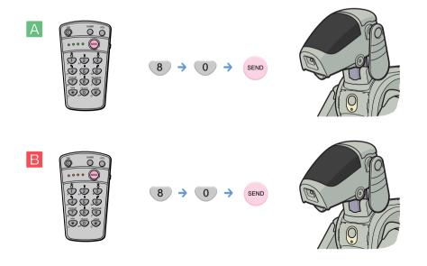
**3** For each command type, press the GAME button and set each AIBO to the game mode. The controller lights and eye lights flash in green for command type A and in orange for command type B.
